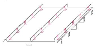
In all wind zones, it is Steelformers standard practice that the clips are to be fixed to all ribs of all purlin lines (or nog/girt lines for wall applications).
