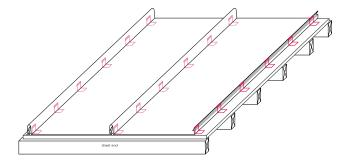
In all wind zones, it is Steelformers standard practice that the clips are to be fixed to all ribs of all purlin lines (or nog lines for wall applications).
